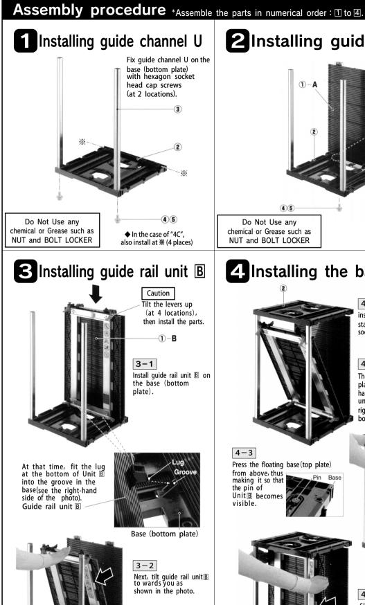
3 Installing guide rail unit B
