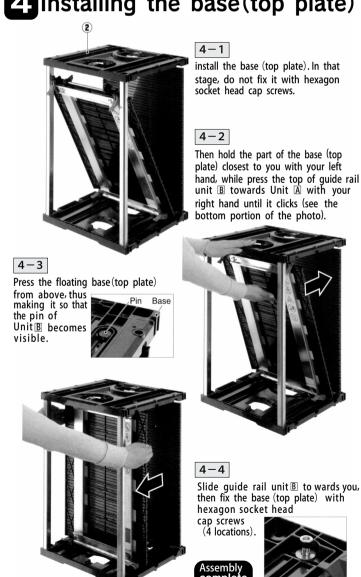
Tightening tool: Hex wrench (2-sided width: 5 mm), tightening torque: 2.70 ± 0.25 N ⋅ m (2.45-2.95 N ⋅ m)
